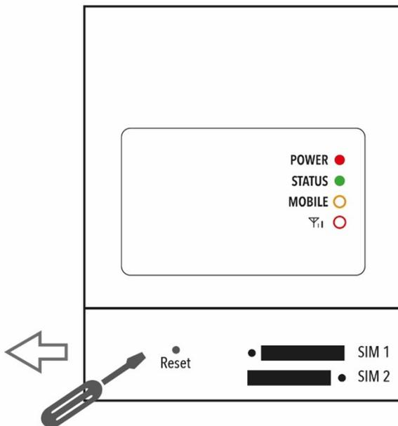
3. After a few seconds, the **Status** LED light will stop glowing. Now press the **RESET button** again:
