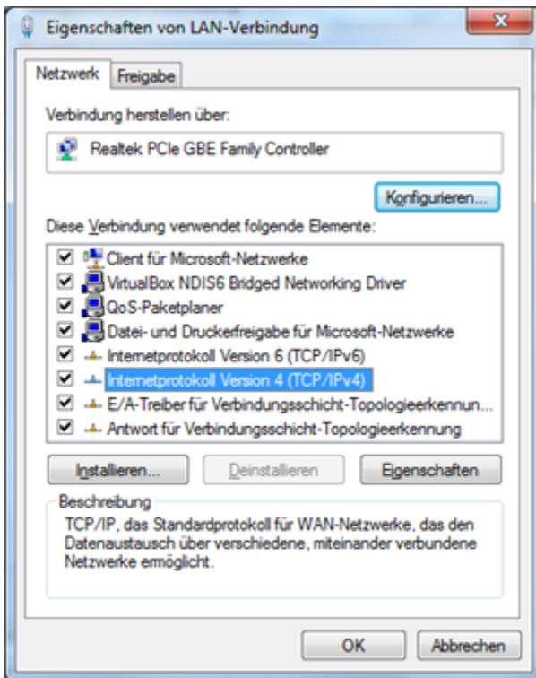
1. Select “*Internet Protocol Version 4 (TCP/IPv4)*”, click the “*Properties*” button, and check if your PC can obtain IP and DNS address automatically. (You can also set up the PC in the subnet: 192.168.2.0/24, e.g. IP: 192.168.2.10, netmask: 255.255.255.0, default gateway: 192.168.2.1)
