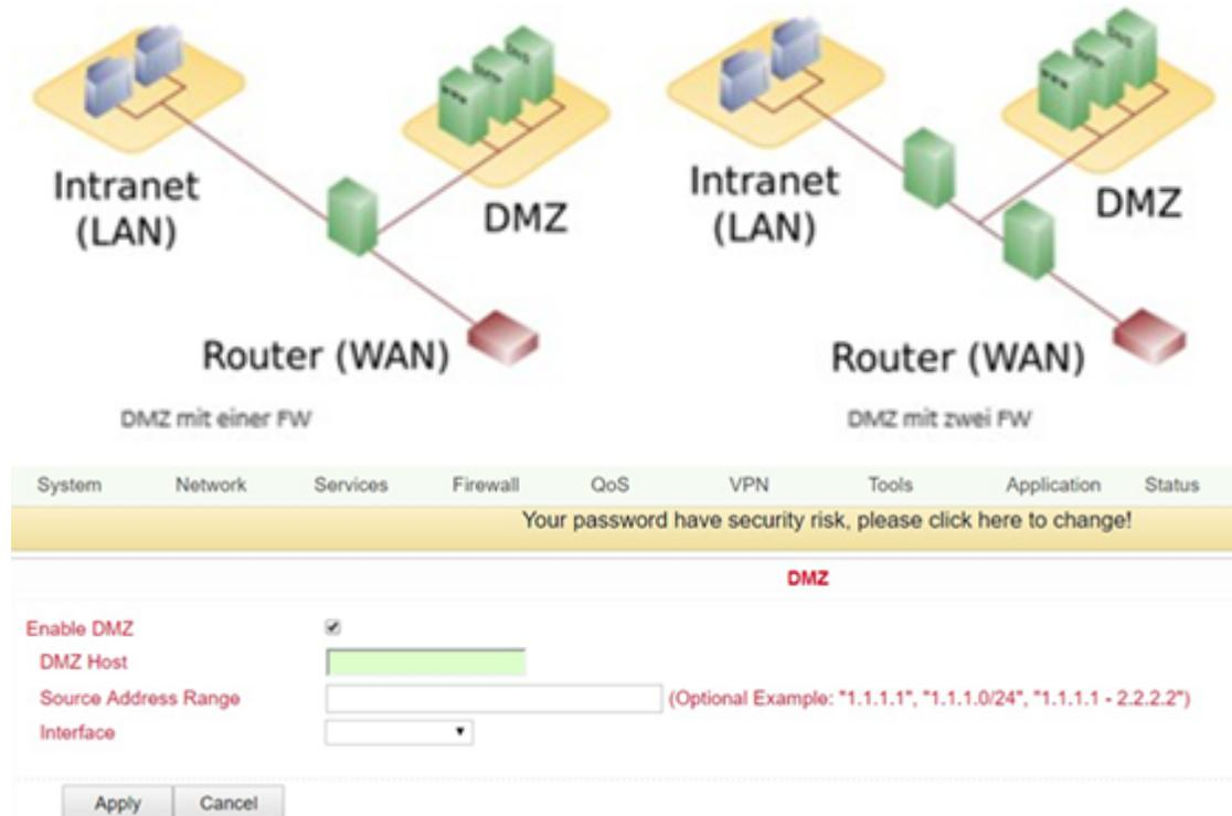
By mapping all ports and the external PC, you can access all ports of the device connected to the TK100.
