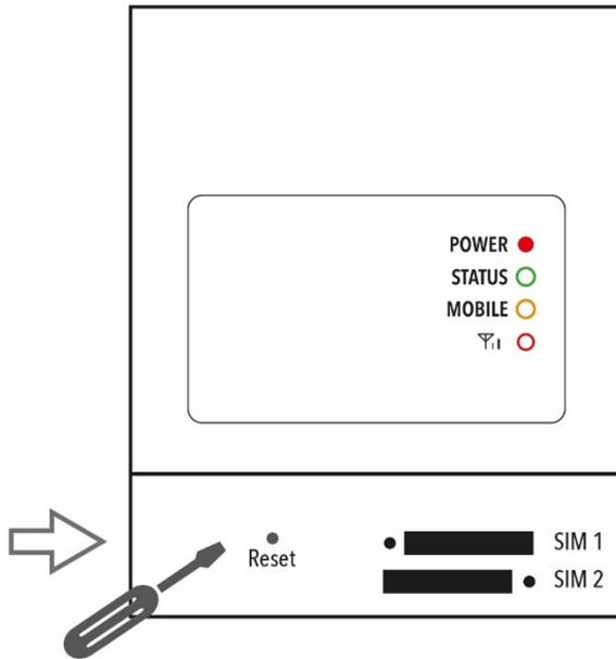
2. As soon as the **Status** LED lights up (approx. 15 seconds after switching on), release the **RESET button**:
